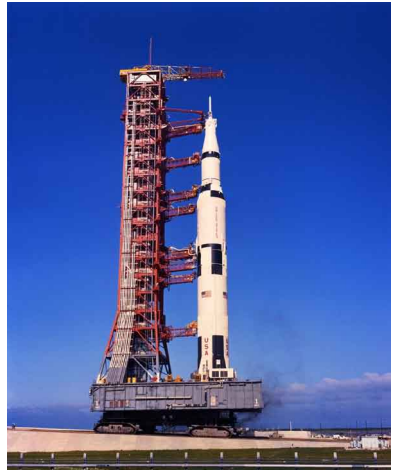
Big Brother a Saturn V (there were no Saturns 2-4) on the launch pad. The prominent black markings made the rocket easier to track against a bright sky.
