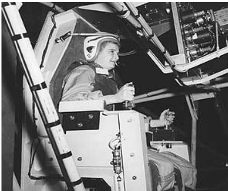
Jerrie Cobb being tested in the Gimbal Rig, a device used to test the ability of a pilot to control the spin of a tumbling spacecraft.
