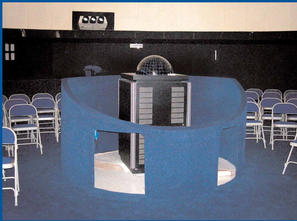
The Digistar 2 projector sat in the centre of the Theatre and used a fisheye lens to project the starfield
